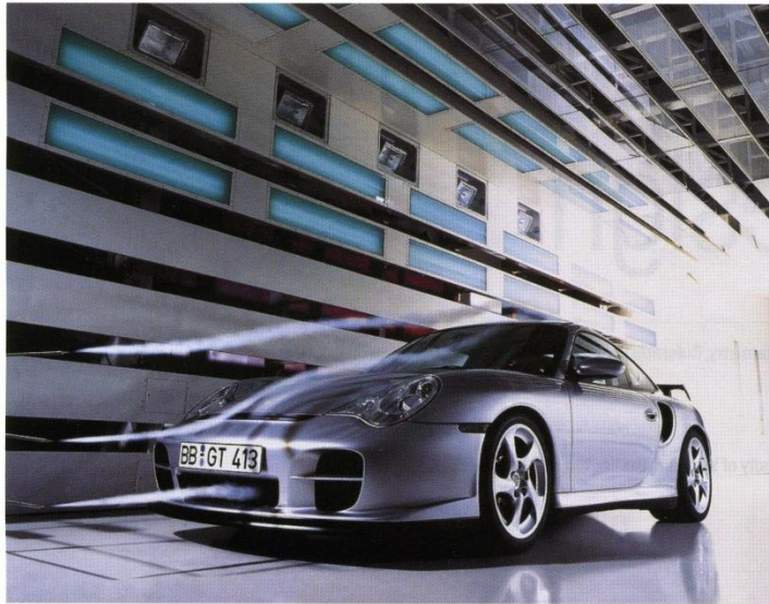
Figure 1 2002 Porsche 911 GT2 coupe in a wind tunnel. The lamellar flow of the smoke along the hood is a visual indication of a low aerodynamic drag.
