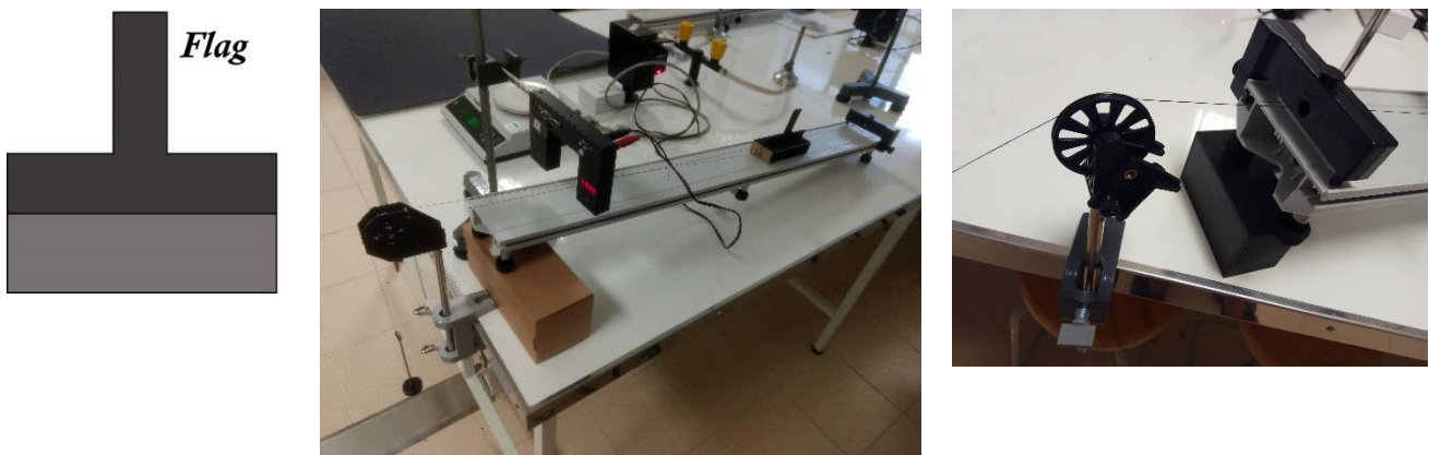
Fig. 3. Experimental assembly: (left) skate and (right) assembly with the photoelectric cell.
